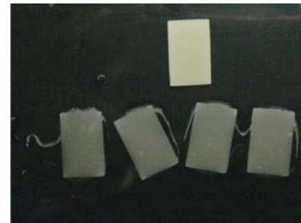
Figure 1. A specimen (top) from the same ceramic group is on the black background without glycerin. The remaining ceramic specimens (below) are sitting on a black background using glycerin as coupling medium.
