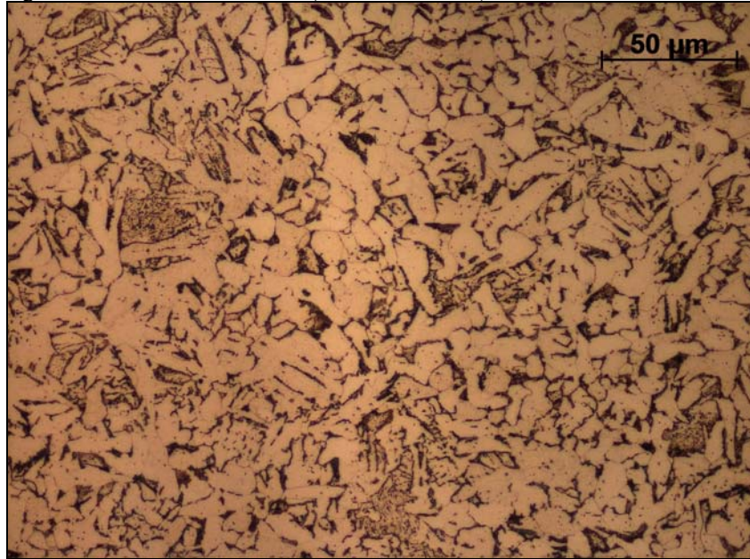
Figura 4.2 – Micrografia metal base ASTM A36 (500X – Nital 2%)
