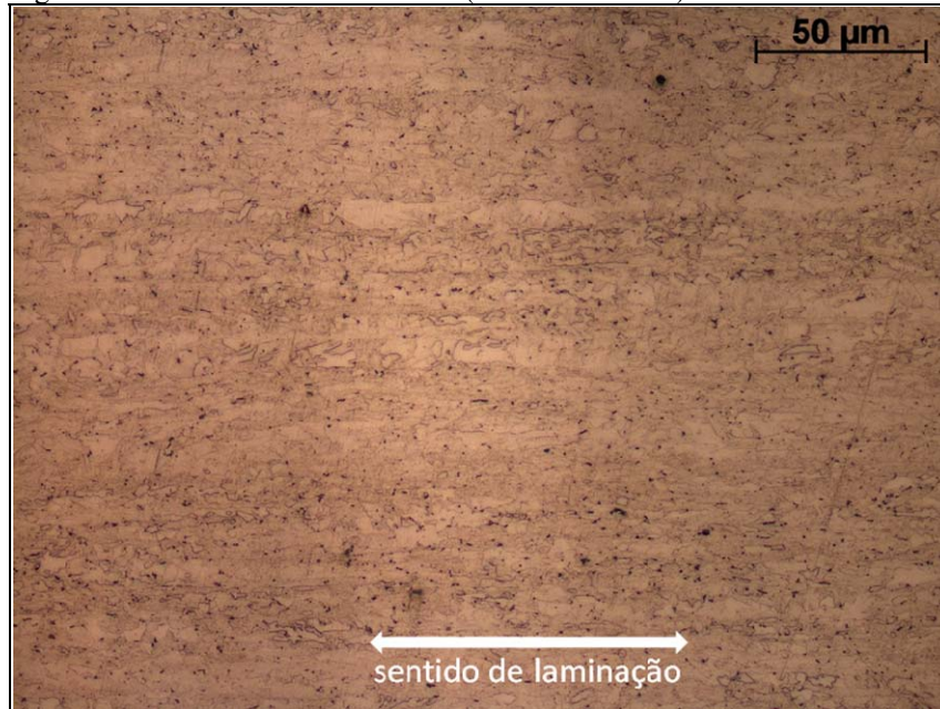
Figura 4.5 – Micrografia metal base DOMEX 700 MC (500X – Nital 2%)
