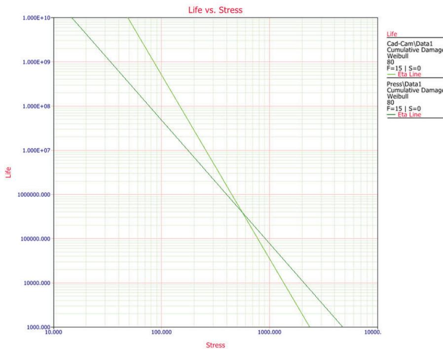
Figure 2. Life (cycles) vs. Stress (N) graph comparing the experimental groups after fatigue test.
