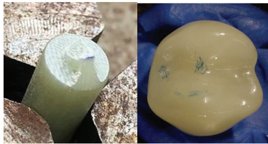
Figure 1 – Loading pistons preparation: (A) Piston design to fit the half of the pre-molar crown (B) Occlusal marks from the three-point occlusal contacts (tripodism) between the ceramic crown and the epoxy resin piston.
