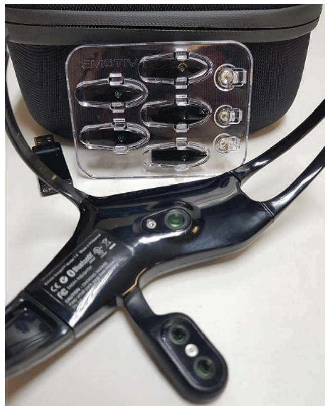
Figure 5. Emotiv Insight and its electrodes.
