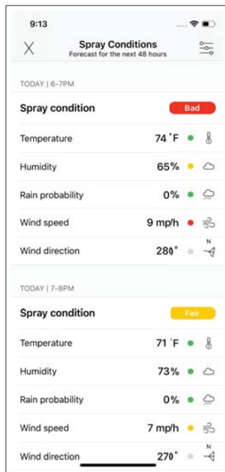
(a) SAS Pro: Bad and Fair spraying conditions due to high wind speed values.
