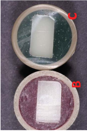
Figure 7 A– Polishing machine for polishing of Cs. Cs aspect before (B) and after (C) polishing the surface.
