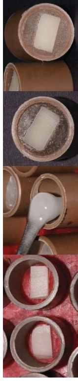
Figure 6. Sequence of inclusion of cs in acrylic resin, leaving exposed only the surface to receive one of four experimental adhesive treatments, prior to direct bonding of orthodontic brackets.
